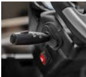
Self cancelling integrated turn signals
