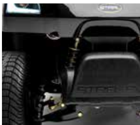
Independent suspension with double A-arms
